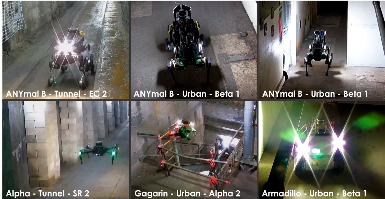
Figure 1: Instances of deployments of the CERBERUS robotic system-of-systems in the DARPA Subterranean Challenge Tunnel and Urban Circuits. Upper row: ANYmal B on wheels and two standard ANYmal B robots exploring sections of the Tunnel Circuit’s “Experimental” Course and Urban Circuit’s “Alpha” and “Beta” Courses. Lower row: the Alpha and Gagarin Aerial Scouts in the Tunnel Circuit’s “Safety Research” Course and the Urban Circuit’s “Alpha” Course respectively, alongside the Armadillo rover in the Urban Circuit’s “Beta” Course. Relevant video results are available at http://bit.ly/cerberus2020
