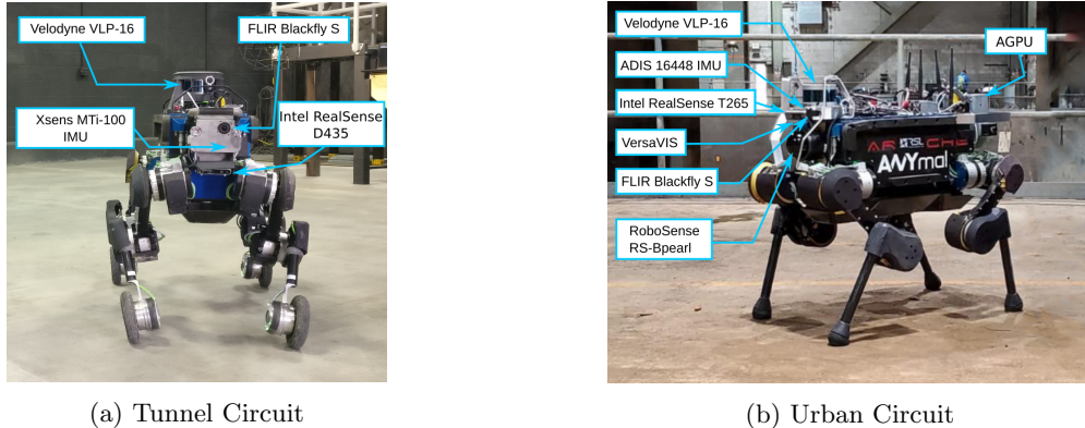
Figure 3: ANYmal B SubT robot with specialized hardware and computation payload for deployment in underground settings.
