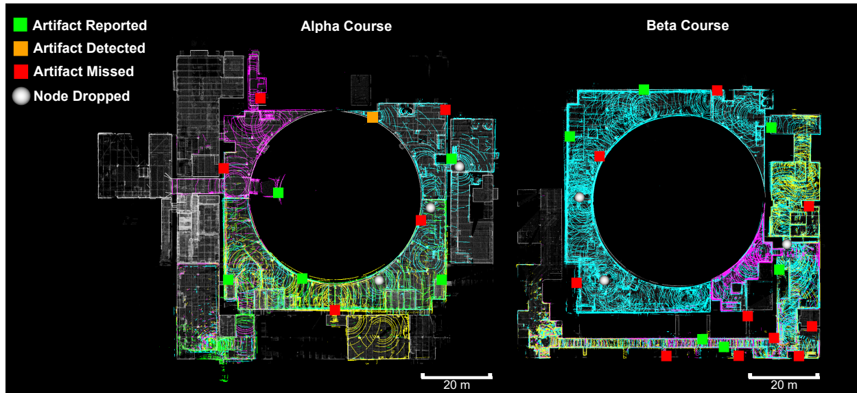
Figure 24: Global multi-robot map of all four sessions of the Urban Alpha and Beta Course using the M3RM approach. The global maps consist of the individual robot maps from ANYmal Bear (cyan), ANYmal Badger (yellow), Armadillo (magenta), and Alpha Aerial Scout (green) if available. Gagarin’s map navigating to the next level is not merged. The ground truth map is denoted in white. The color squares denote successfully reported, detected, and missed artifact locations. The spheres illustrate WiFi beacons dropped by ANYmal Bear.
